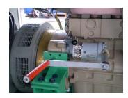
Kineteco's starters are very simple and affordable, making hand starting the smart option on a wide range of machinery. Fitting is easy. Just remove the electric starter and its connectors and bolt on the spring starter.
